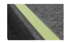
Plate profile made of anodized aluminium with a photoluminescent strip that serves as a guide in case of sudden absence of light. It can be installed as a flooring separator, in entrances, stairs or ramps and also as
