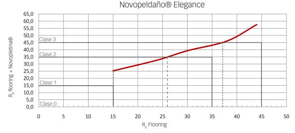
\* In this graph you can see the comparison between the Rd of the flooring without Novopeldaño®Elegance and the Rd of the flooring with the profile installed. The different areas that conform different classes have been delimited to see clearly the improvement obtained of Rd and of flooring class.
