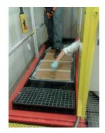
We have tested our Novopeldaño® Maxi under the DIN 51130 standard, to certify its good properties of slip resistance. This reference had been already tested before under the Spanish standard UNE-ENV 12633:2003, which is the one required by the CTE (Spanish Technical Building Code).
