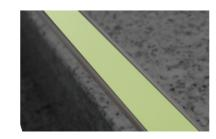
Plate profile made of anodized aluminium with a photoluminescent strip that serves as a guide in case of sudden absence of light. It can be installed as a flooring separator, in entrances, stairs or ramps and also as a luminous guide in walls.
