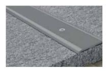
Novo**pletina® aluminium** is a striated plate profile made in anodized matt silver aluminum designed to be installed in stairs, ramps or in areas where the safety against falls wants to be assured. This highly resistant profile is delivered with countersunk holes and is easy to install on finished floorings by using fixing screws.
