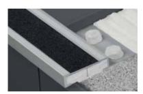
Stair nosing profile made of anodized aluminum, to be installed during the tiling. This profile has a non-slip strip which helps to fulfill accessibility requirements and improves the slip resistance value of the flooring.
