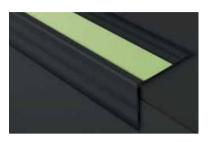
Stair nosing to be installed after tiling work, made of anodized aluminum silver matt finish. This profile has a luminescent strip useful as a guide in case of sudden darkness. With striated surface, it is light and easy to install after tiling.
